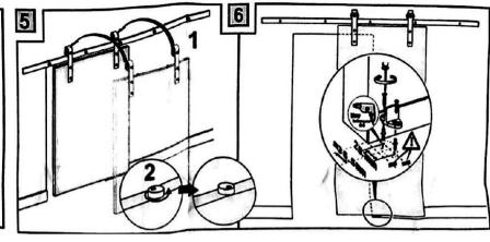
The Fourth step: Install the antioff block. Fix the anti-off block on the top of the door leaf with the screw.
