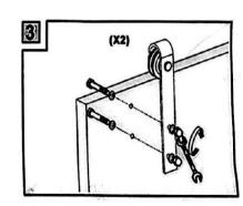
Note: Be attention the level of the hole. The depth of the hole should be 5-7cm.
