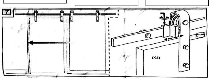
The seventh step: Install limiter Fix the limiter after adjusting the moving distance.
